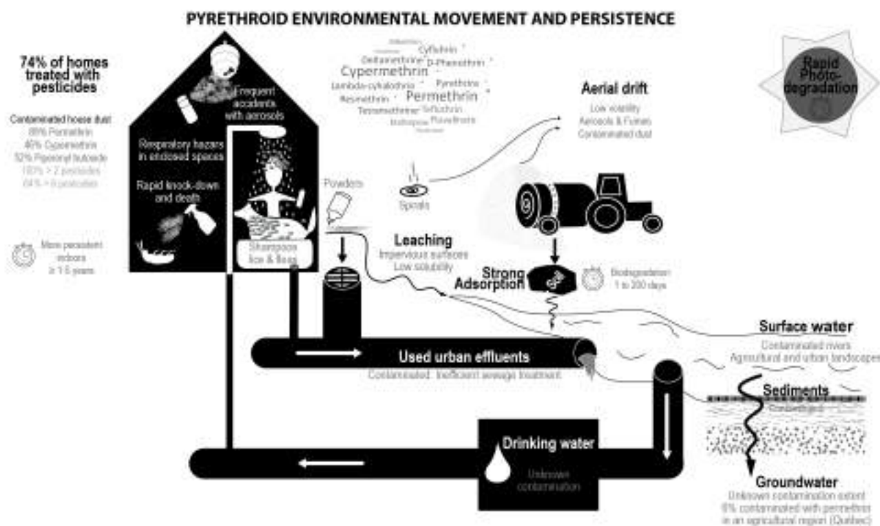
Figure 4: Transport and persistence of pyrethroids within buildings and in the outside environment.
